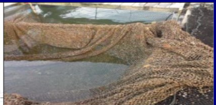
Net exposed to ASM ultrasonic device – 8 weeks after cleaning – no or very little fouling evident.
